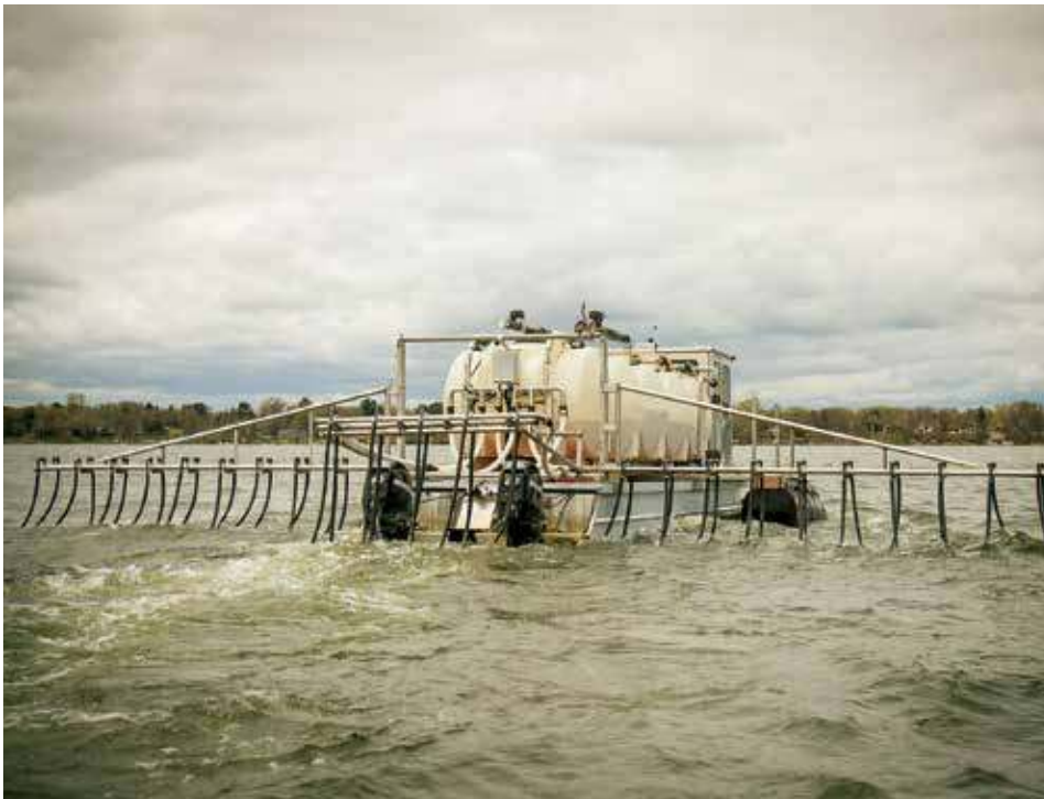
Figure 8. HAB Aquatic Solutions' alum application vessel used to precisely apply alum to Bald Eagle Lake at the prescribed alum dose.
